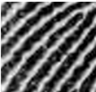
Section of the same fingerprint image that has been compressed 15:1 with the WSQ algorithm. Note the absence of the block artifact. The image has been zoomed by 4
