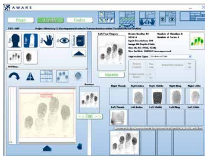
Step 2 - Assembly. This stage allows the operator both automated and manual options to analyze and process the biometric images so that they are of acceptable format and quality.
